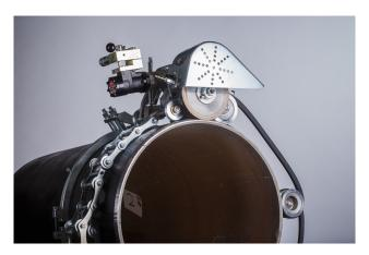
The machines are powered by a hydraulic power pack allowing the blade to track automatically around the circumference of the pipe wall at a cutting speed of approximately 140m per minute. One of the many benefits of the Keel Cutter is that minimum clearance is required around the pipe, only 200mm to 250mm depending on the model, thus reducing size of excavation.
