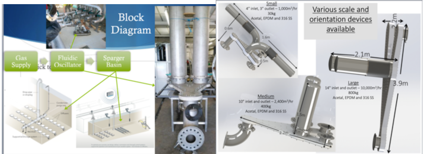
Figure 1 A blower is used to supply the gas. Typically, sparger basins seen below (in different combinations or types – typically EPDM rubber with membrane slits or ceramic spargers) are utilised to provide the aeration requirement. The proxy for measuring this aeration is termed as the mass transfer coefficient (MTC). The higher the MTC, the faster is the rate, and therefore the blower use (power) is reduced. The fluidic oscillator is introduced in between the blower (air-supply) and sparger basin, increasing the MTC, and therefore reducing the energy utilised. Different scales and sizes can be designed and implemented seen in picture on right.
