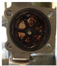
The installed unit and the damage done to the membranes by hydrocarbon contamination.
